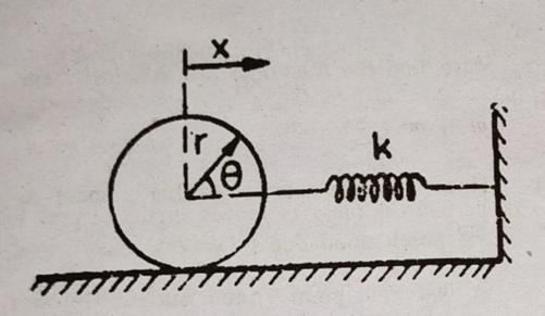
Determine the frequency of horizontal oscillations of the system if the cylinder:
